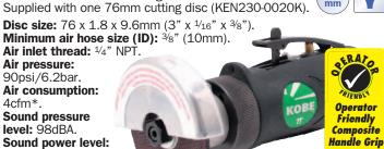
103dBA. Vibration level: 0.5m/s<sup>2</sup>. Overall length: 185mm.
